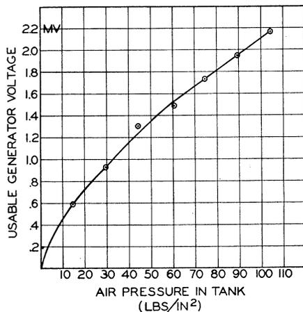
FIG. 1. Curve showing maximum usable generator voltage as a function of air pressure in the enclosing tank. Air pressure is given in lb./in<sup>2</sup>, absolute (not above atmospheric).
